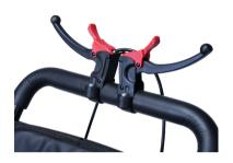
To brake the wheelchair, first pull the brake levers at the back of the chair and then push it upwards until you hear a "snap," indicating the brake is engaged. (shown in the image above)
